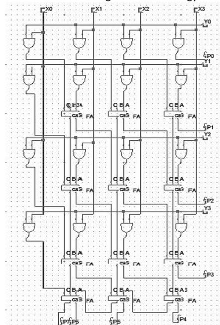
**Fig.3 Schematic of the 4 bit array multiplier using DSCH 3.5 tool**
