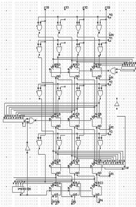
Fig.5 Schematic of the 4 bit array multiplier with power gating technique using DSCH 3.5 tool
